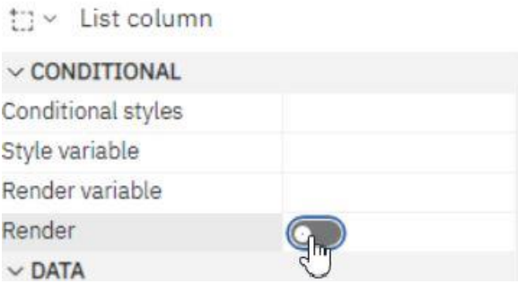
Figure 503 - Hide column in reports -List column properties - Conditional - Set Render to No
