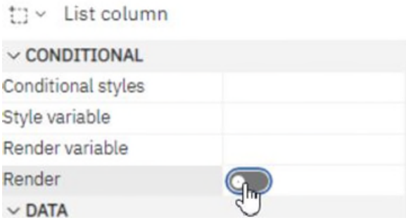
Figure 428 - Hide column in reports -List column properties - Conditional - Set Render to No
